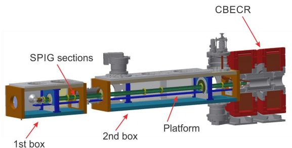
Fig. 1. Engineering representation of the new SPIG assembly together with the Charge Breeding ECR [1].
